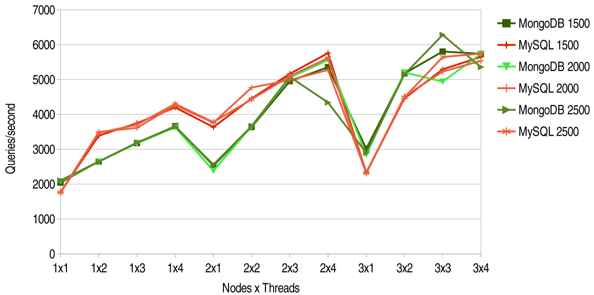
Figure 4.3: Multiple benchmark configurations with simple query measuring queries/second with larger number of queries
