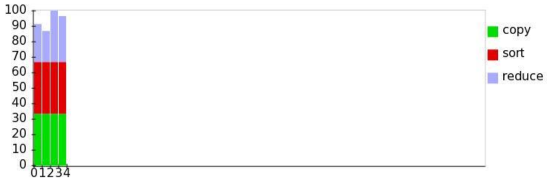
Figure 31: An example of reduce task execution indicating the three phases Copy, Sort and Reduce.
